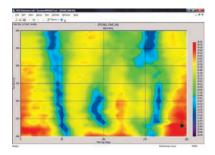
Test Data Output TDK Emissions Lab allows you to view test data in a table as well as in many different types of graphs: x-y plot of amplitude vs. frequency, colored contour plot of amplitude vs. antenna height and turntable position, polar plot of amplitude vs. turntable position, and x-y plot of amplitude vs. antenna height.
