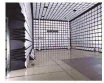
levels inside the chamber. NSA deviation is guaranteed to be within  $\pm 3.5$  dB for a test volume of 4 m Æ, 2.5 m high. By positioning TDK ferrite tile floor plates and IP-045C absorbers between the transmit antenna and EUT (Equipment Under Test), the semi-anechoic chamber can be used to perform radiated immunity measurements in full compliance with IEC 1000-4-3 standard in the frequency range from 26 MHz to 18 GHz.
