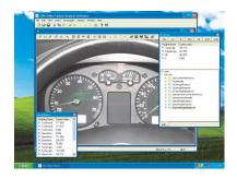
Video Capture The Video Capture option in TDK EUT Monitoring Lab allows you to use a camera to detect EUT events during an immunity test, as well as to record video of the entire test for later playback and observation of EUT events. It offers great flexibility in the definition of the types of changes in the video image that constitute an EUT event.
