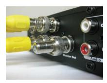
Connect a BNC to RCA connector to the MONITOR OUT connection on the back of the DVR.
