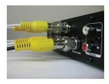
Plug the RCA cable into the BNC connector.
