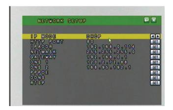
**HTTP Port**: Refers to the port that your DVR will use to communicate with your network and the Internet. This port is required to be entered at the end of the IP address to connect to the DVR. (Ex. If using port 2000 and the IP address is 192.168.1.103 you would type http://192.168.1.103:2000 in the address bar of I.E.) If using port 80 your Internet browser will automatically add it in at the end of the address, even though it may not be visible.
