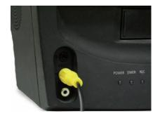
Attach the other end of the RCA cable to a yellow RCA video input on your monitor.
