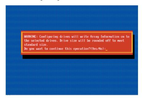
**6.** Make sure that you have selected the correct disk drives to configure. If correct, type **Y** to continue.
