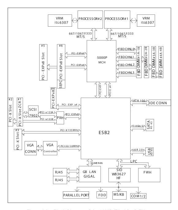
Figure 1-9. Block Diagram of the 5000P (Blackford) Chipset
