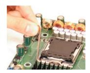
Plastic cap is released from the load plate if the CPU is properly installed.
