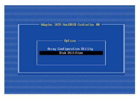
**1.** From the Adaptec RAID Configuration Utility Menu, select **Disk Utilities** (as shown above) and press **<Enter>**. The following screen appears.
