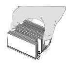
3. Once the CPU is loosened, remove the heatsink from the CPU socket.
