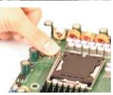
2. Gently lift the load lever to open the load plate.
