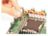
Load Plate \_\_ (with PnP Cap attached)
