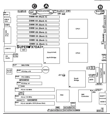
A. 24-pin ATX PWRB. 8-pin Processor PWRC. 4-pin PWR
