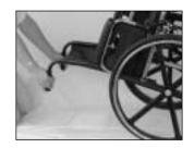
c. Lift caster post assembly out of existing position and insert in top mounting hole position.
