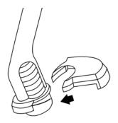
**Note**: A guide rail and a hook are on the lower part of the motor casing (7), left and right. The protective shield should be pushed forward from the rear onto the guide rail until the hooks engage.
