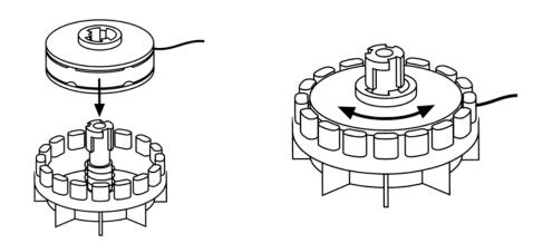
6. Replace the tap button and press it gently down against the spring. Turn the tap button in a counterclockwise direction until it latches tightly.
