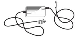
**Recharging time for the battery is approximately 5-8 hours**. The charger light, which glows red when the battery is not fully charged, will glow green when charging is complete.
