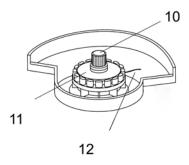
Hold the cutting head with one hand and press the tap button down with the other hand. At the same time, turn the tap button in a counterclockwise direction. Remove the tap button.
