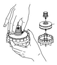
**Note**: If the tap button cannot be pressed down, turn the cord cartridge to the right or left until it stops. Then proceed as described above.
