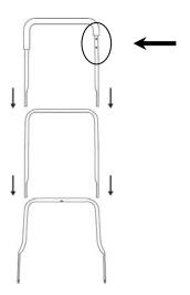
4. Attach the two-handed safety switch to the top section. Run the cable along the top side of the handle (so it does not hang down behind the mower) and close the "clamshell" portion of the safety switch around the screw holes. Fasten by inserting and tightening the two screws provided.
