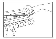
5. Make the same adjustment at the other end of the cutting bar.
