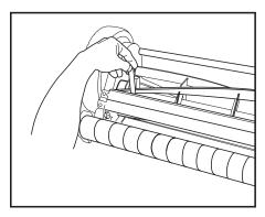
7. The blades may also be tested by inserting a piece of paper vertically into the blades while turning them by hand.
