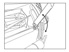
3. Continue assembly of the middle and top sections of the handle using the handle bolts and wing nuts. The top section must be attached with the two holes near the grip area on the right side (standing behind the mower).
