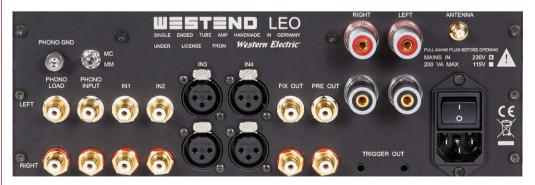
The connection panel offers sufficient possibilities to connect external sources. The XLR inputs are debalanced immediately; a Class A circuit is always unbalanced. Gold plated sockets – as befits this price range. The standby switch is located at the front and the mains switch at the rear.
