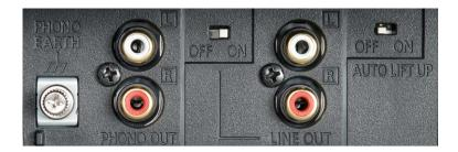
If you want to use the phono input on the amplifier, use "Phono Out" (I.). If the internal phono pre is activated, the cable belongs to "Line Out" (r.). "Auto Lift" lifts the scanner out of the groove at the end.
