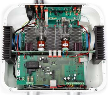
Neatly constructed with the necessary thermal space. The output transformers are designed as toroidal cores and equipped with heat sinks.
