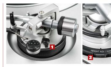
The meticulously crafted aluminum tonearm is extremely smooth-running and can be adjusted in height after releasing the locking lever **1**. Those who frequently change the cartridges can orient themselves on a scale **2**.
