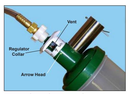
Figure 17. Oxygen Concentration Control
