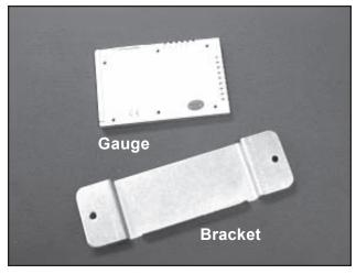
Figure 25. Rear View of the New-style Gauge (removed from door)
