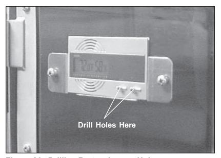
Figure 26. Drilling Button Access Holes
