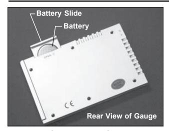
Figure 14. Gauge Battery Slide and Battery
