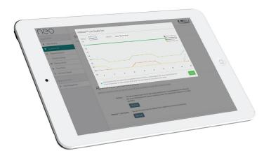
With our monitoring platform, neo will report on the cable and termination quality for every HDBaseT™ link. It's possible to find out where in a cable run the problem is (how many meters along) or which one (or more) of the pairs are not terminated correctly. This can save hours of wasted investigation, what's better is its all free and available across our entire product line.
