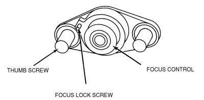
THE CENTER SECTION of the control is a threaded member that focuses the bulb in relation to the reflector. Turning this adjustment moves the bulb on the horizontal plane, into or out of the reflector. Rotating this section clockwise moves the bulb away from the reflector. The small knurled screw to the left of this section can be tightened to lock the focusing mechanism in place after the bulb alignment procedure has been completed.
