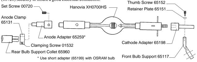
REMOVE THE PLASTIC PROTECTIVE COVER from the xenon bulb only if necessary. Insert the bulb through the top of the lamphouse, between the reflector support and the front casting. Pass the anode (+) end of the bulb through the hole in the reflector, taking care *not* to touch the surface of the reflector.
