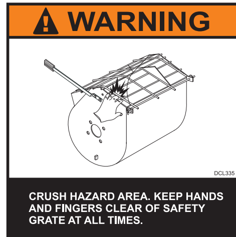
Figure 37. Safety Grate (Crush Hazard)
