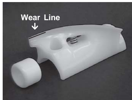
Figure 12. Auger Flight Wear & Front Auger Support Bushing Wear
