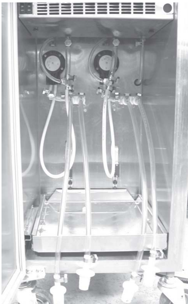
Figure 9. Completed BCS Hose Assembly
