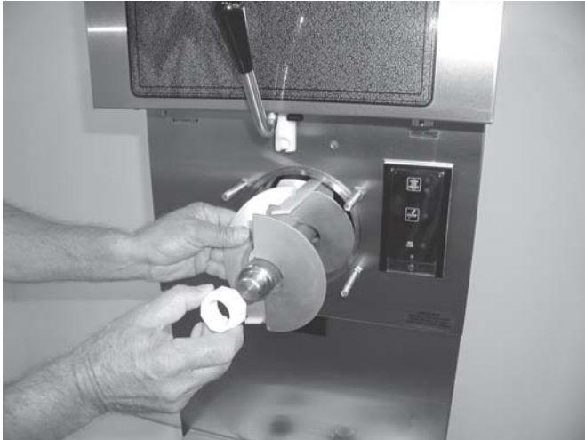
Figure 18. Auger Shaft Removal
