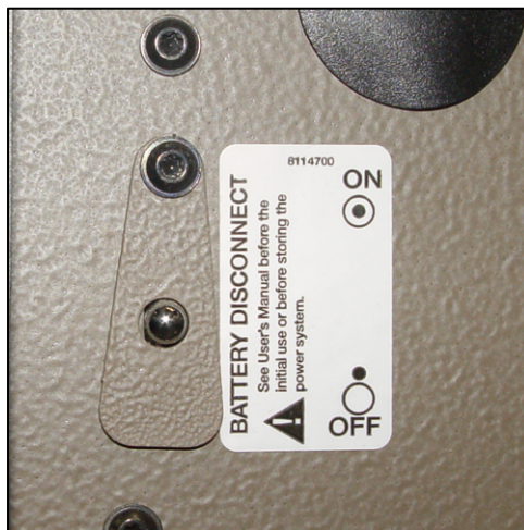
Power output disconnect switch location
