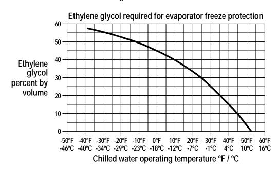
Figure 3 Freezing Protection Curve
