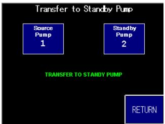
**Note:** When you enter the second pump number, the controller checks to make sure that both pumps are offline and that the standby pump has no stations assigned to it.
