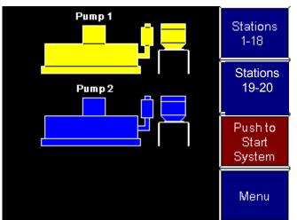
Figure 14: "Pump Status" Screen During Operation
