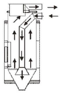
Figure 3: Drying Hopper
