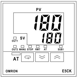
**Note:** The only functional buttons on this contoller are the up and down keys.
