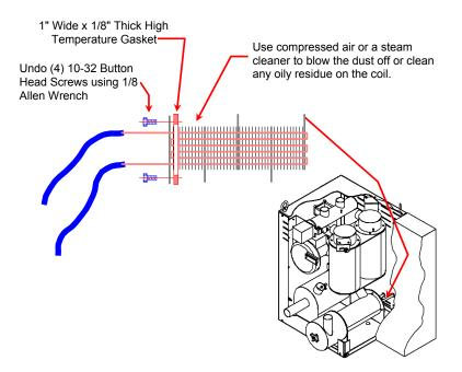
Note: To clean the cooling coil, use compressed air or a steam cleaner to blow the dust off or clean any oily residue on the coil.
