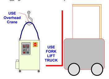
Note: Floor Mounted Dryers can be lifted by hoist or fork lift.
