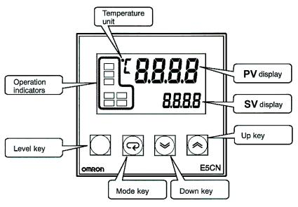
**Identifying Process Air Temperature Controller LED Indicators**
