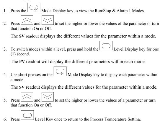
Figure 6: Settings for Process Temperature Controller (E5CN), Part No. A0555757
