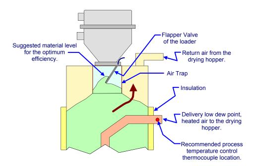
Figure 1: Drying Hopper Air Trap
