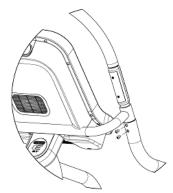
(e) Position the lower end of the left handrail over the rear leg weldment, then pulling the handrail towards you secure it into position with 2 washers and 2 hex screws provided using a 5/32" (4mm) hex key or T-handle.
