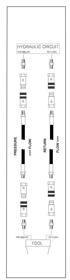
Figure 1. Typical Hose Connections
