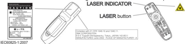
[Class2 Laser Product] Wavelength: 650nm, Maximum Output: 1mW, No beam divergence [Laser Diode] Wavelength: 650nm, Maximum Output: 6mW, Beam divergence: 30deg(perpendicular) / 8deg(parallel)
