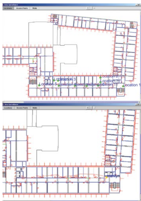
Figure 5. Indoor location determination using WiFi fingerprinting with the system 'ipos' on the 3rd floor of our office building (on the top the location of the calibrated points is shown and on the bottom the trajectory of a moving user along the corridor)
