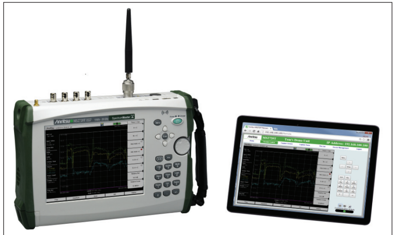
Figure 1. The MS2720T Spectrum Master with Anritsu's Web Remote Control Tools being controlled from a tablet.
