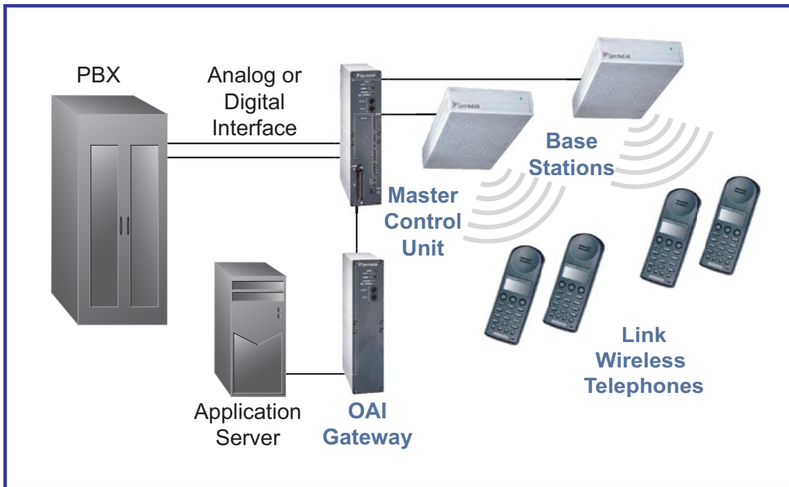
The Link Wireless Telephone System
