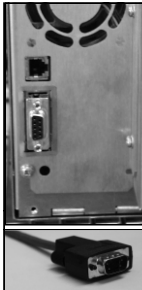
Figure 3-9 Copper cable and DB-9 connector.
