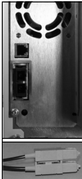
Figure 3-8 Optical cable and SC connector.
