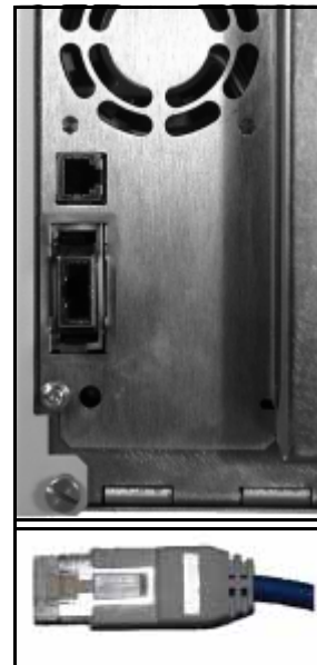
Figure 3-10 Copper cable and HSSDC connector.
