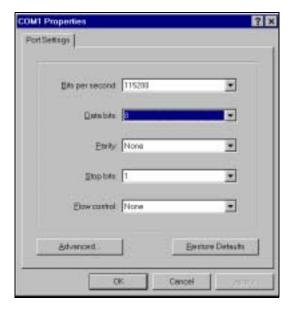
Figure 11-11 Serial port settings.
