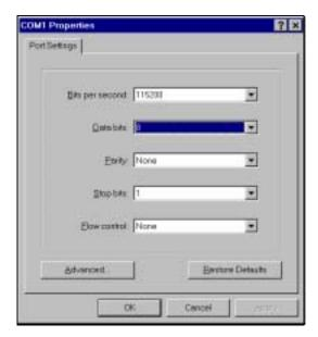
Figure 7-1 Serial port settings.
