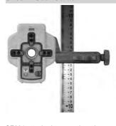
SF601 attached to a grade rod using the standard receiver clamp
