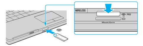
Be sure to hold the Memory Stick media with the arrow pointing in the correct direction as you insert it into the slot. To avoid damaging your computer or the Memory Stick media, do not force the Memory Stick media into the slot if you cannot insert it smoothly.
