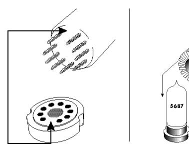
Note the larger space between two of the pins and holes for proper alignment of tube and socket.
