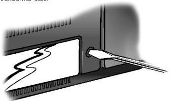
The location of the screw which locks the tube cover in place.
