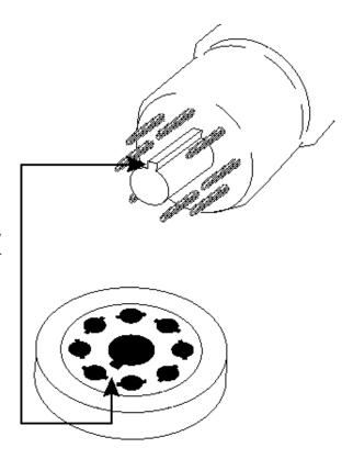
Note the locating center key and notch for proper alignment of tube and socket.
