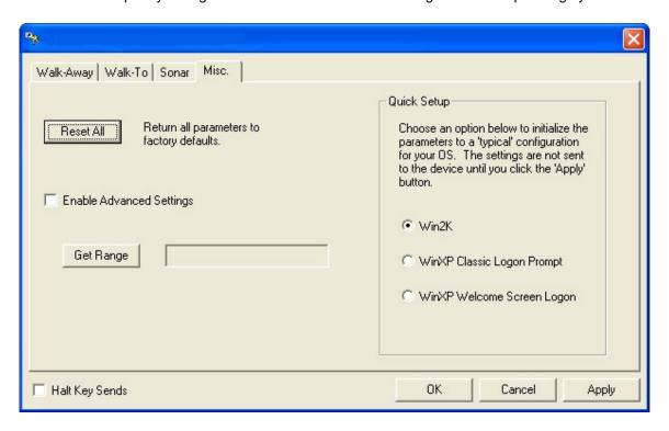
Figure 5: Misc. folder for Quick Configuration of Walk-To and Walk-Away Keystroke Settings
