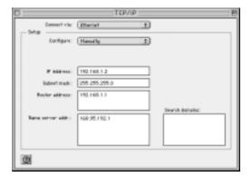
Figure 25. Manual Configuration of IP Addresses
