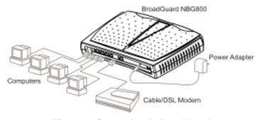
Figure 4. Connecting the BroadGuard
