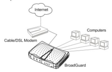
Figure 1. BroadGuard Connections
