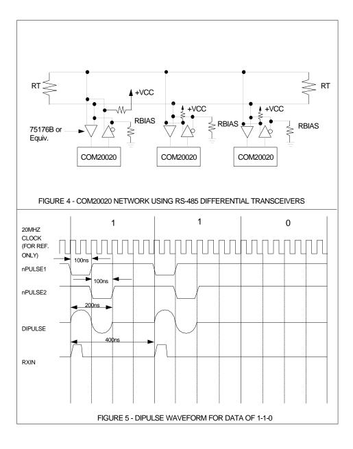
In typical applications, the serial backplane is terminated at both ends and a bias is provided by the external pull-up resistor.
