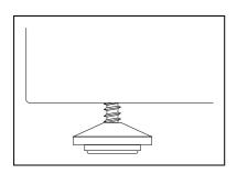
Two spacers attached to the appliance must be fitted onto the upper edge of the condenser, thus preventing the appliance from being installed too close to the wall. Spacers are manufactured for all-purpose function depending on the distance of the condenser from the wall. Therefore turn spacers correspondingly and fix them to the appliance.
