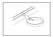
From time to time wipe the condenser on the rear wall with a soft non-metal brush or vacuum cleaner.
