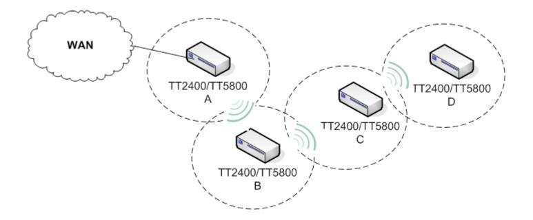
In this configuration setup example you'll be expanding your wireless network coverage that will span an area in length.
