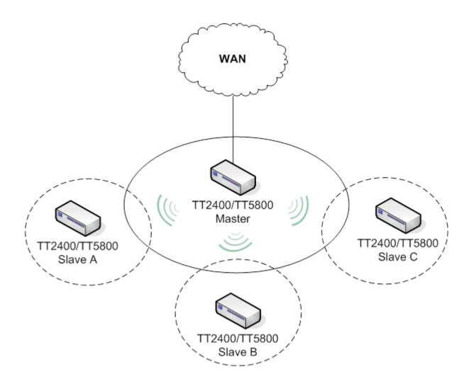
This is the mode to use if you're expanding the hotspots in the area around your master AP that is connected to the WAN. What you'll need to do is enable WDS and ACL on all the APs. Then input each of the MAC addresses of Slave A,B,C into the Master AP under both the WDS and ACL section. For the Slave APs A,B,C you'll input only the MAC address of the Master AP into the WDS and ACL list to limit them to direct their traffic through the Master AP only.
