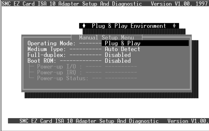
Figure 2-2. Manual Setup - Plug and Play Environment
