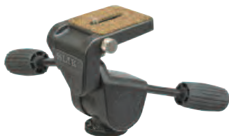
SH-908 618-908 Heavy Duty 3-Way Pan Head with smooth precise movements Height: 5.31 in. Weight: 3.00 lbs. Max.Operating Load: 22.00 lbs.
