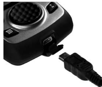
Fig. 4: Inserting the mini-USB connector
