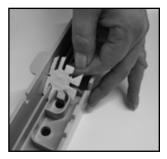
6. Wipe any loose sediment from the water tray. Make sure no particles are allowed to plug the drain hole.
