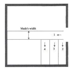
Cut the strips smaller if the floor covering is bonded very securely, e.g. with an epoxy adhesive.
