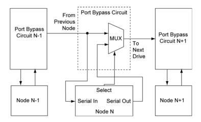
Figure 6. Typical Backplane Bypass Circuit
