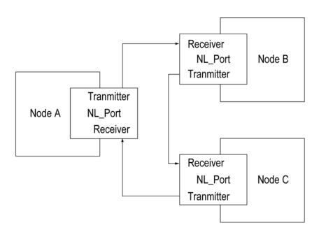
Figure 4. Arbitrated Loop Topology Connection
