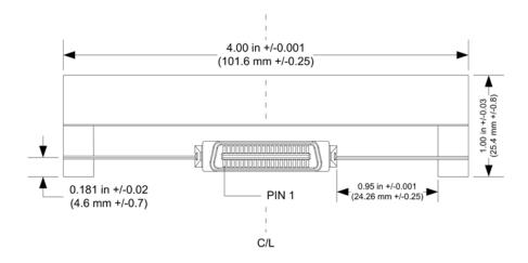
Figure 3. Relative SCA-2 Connector Location
