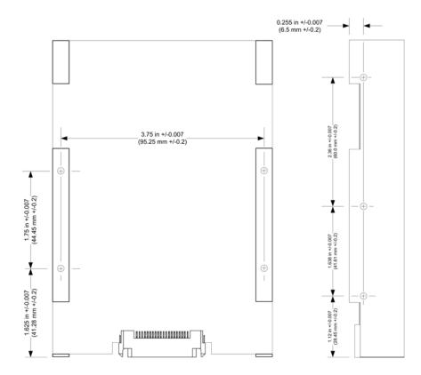
Figure 11. Exterior Mounting Specifications
