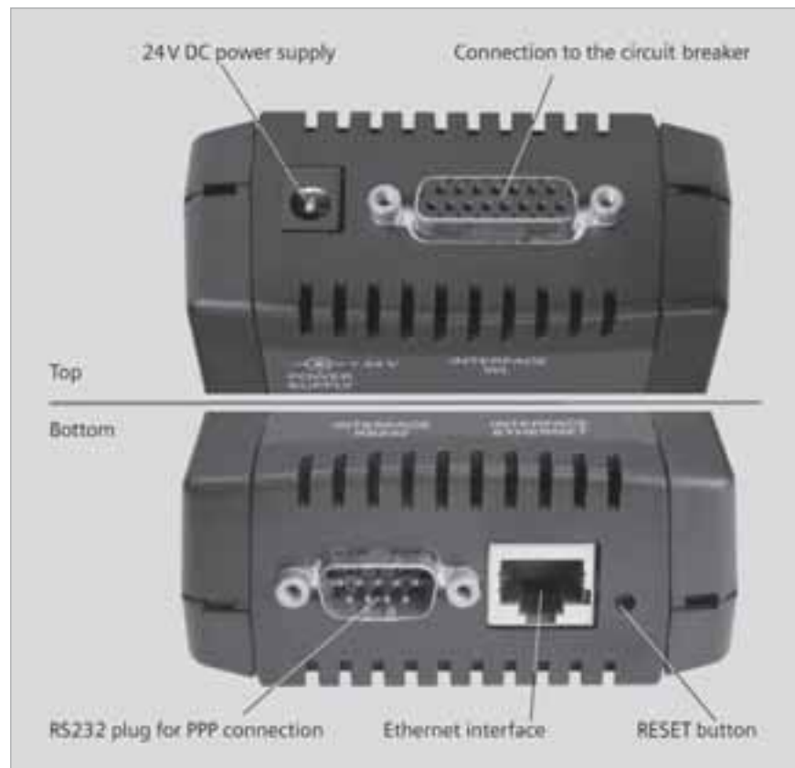
Figure 4-1 The physical BDA interfaces. The connection to the circuit breaker and optional power supply are on the top, while the RS232 interface (or the Ethernet interface in the case of BDA Plus ) and the RESET button are on the bottom.
