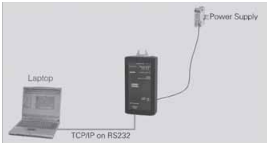
Graphic 4-1 The BDA must be supplied externally with 24V DC. Parameters can be set, stored, and printed out.
