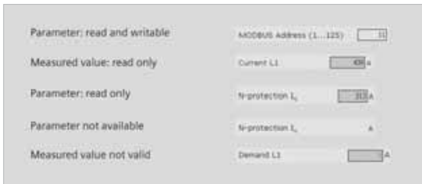
Figure 4-19 The way data is displayed on the BDA pages depends on the property byte. This tells you which data is read only, which data can be written, and which data is not available.
