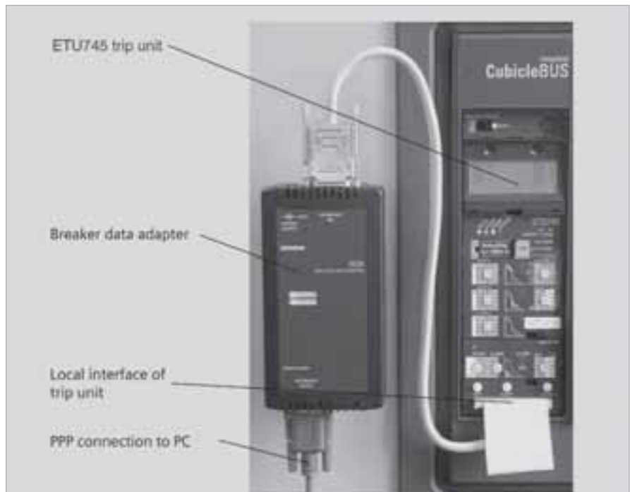
Figure 4-2 For temporary operation, the BDA can be connected to the local interface of the trip unit. In this configuration, only the RS232 connection to the PC is typically used.
