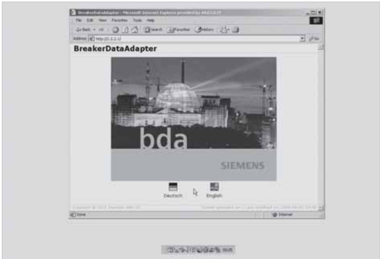
Figure 4-8 Installing a data comm. connection to the BDA with Windows98, part 2 (identical to Windows95 and WindowsME): Once communication has been established, the connection window disappears from the Windows systray. To display the BDA pages, enter address 2.2.2.1 in the browser. To call up the connection window, double-click the relevant icon in the systray.
