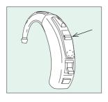
You can adapt to a changed hearing situation by lightly pressing the program button. For instance, you are better able to understand the person you're talking to even in disturbing background noise.
