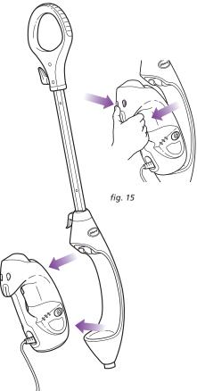
To remove the Handheld Steamer, press and hold down the Handheld Release Buttons while pulling out the Handheld Steamer. (fig. 15)
