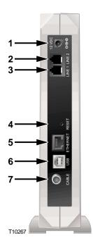
1 POWER - Connects the cable modem to the DC output of the AC power adapter that is provided with your cable modem
