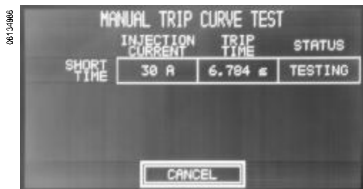
Figure 33: Manual Trip Curve Test Screen
