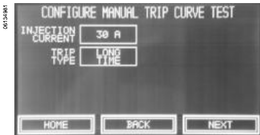
Figure 36: Configure Manual Trip Curve Test Screen
