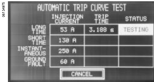
Figure 20: Automatic Trip Curve Test Screen
