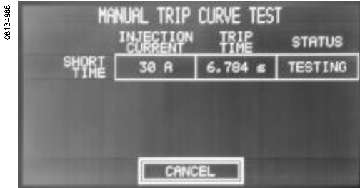
Figure 39: Manual Trip Curve Test Screen
