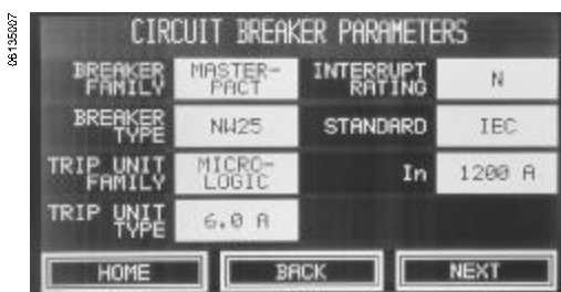
Figure 64: Circuit Breaker Parameters Screen
