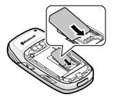
Note: When you need to remove the SIM card, slide it, as shown, and take it out of the socket.
