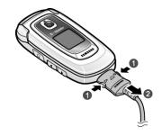
**Important!**: You must unplug the Travel Adapter before you remove the battery from the phone during charging; otherwise, the phone could be damaged.
