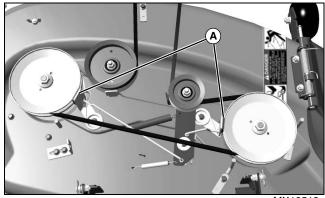
3. Remove left belt shield and adjust two blade brakes (A).
