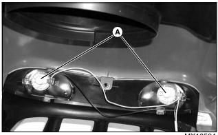
3. Turn bulb socket (A) 1/4 turn counterclockwise to
