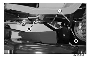
6. Fasten rear draft arms (A), two on each side, with washers and spring locking pins (B).
