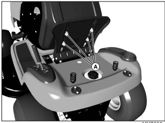
Lubricate plastic washers and bushings (A) under the seat with a general all-purpose spray lubricant.
