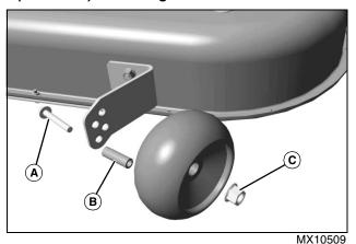
4. Check mower wheel position. Remove bolt (A), bushing (B), and nut (C) and move mower wheels to proper hole.
