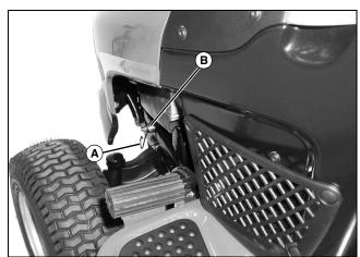
3. Keep hood in the closed position and pull spring hook
