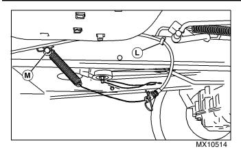
• Push PTO drive cable into clip (L) and hook end of cable spring with hardware (M) into peg on left side of machine frame.
