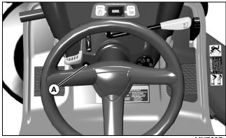
3. Push and hold in the reverse implement switch (A) while depressing reverse foot pedal.
