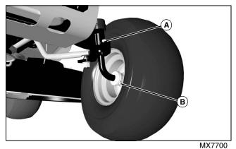
Lubricate front wheel spindles (A) and bearings (B), one
