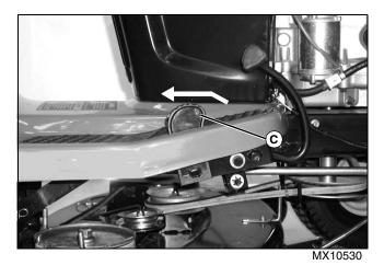
3. Touch the reverse travel pedal (C) with front of foot and slide foot over pedal from front to rear.
