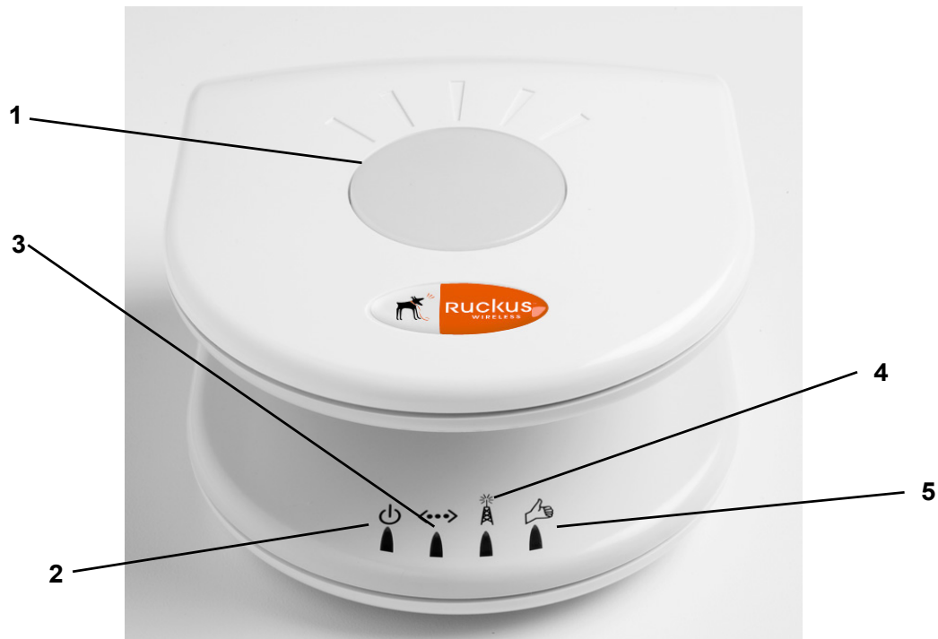
Figure 2—Front View of the Ruckus Wireless 2825 Wireless Multimedia Router
